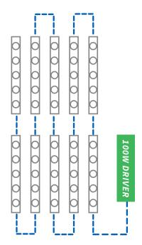
\*\*Please note all LED lights must be connected in series (single continuous loop),
